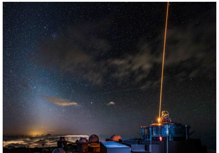
Sodium guidestar for sensing atmosphere at the Maui Space Surveillance System facility atop Haleakala. Photo credit: Robert Q. Fugate
